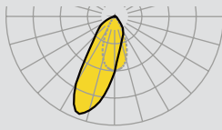
Asymmetrical 5,600-12,600 lm Installation Height: 3-4m
