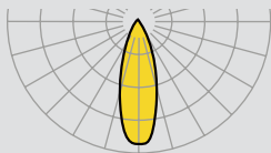
30° 5,600-12,600 lm Installation Height: > 10 m
