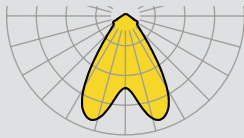
Double Asymmetrical 5,600-12,600 lm Installation Height: 3-4m
